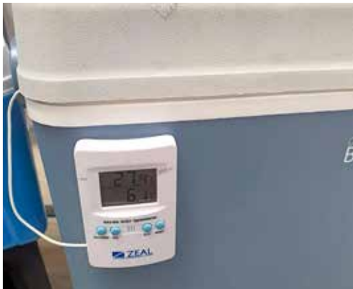
Cold box with built in temperature data logger.
